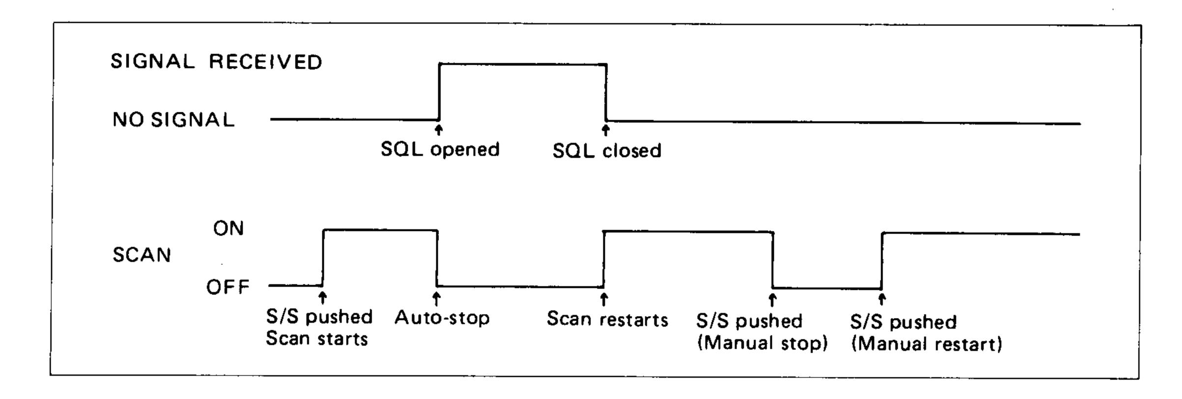
2. By setting the SCAN-STOP TIMER Switch in ON position and the SCAN-STOP FUNCTION SWITCH in BUSY position, the scan will stop on a signal, and will restart after specified time is passed, whether a signal has been received or not. The scan stop time is selectable 3 seconds (SHORT) and 9 seconds (LONG) with the SCAN-STOP INTERVAL Switch located under the access cover.
